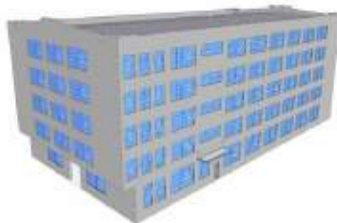
Gambar 3. 21 Ilustrasi Out-of-plane setback Sumber : (FEMA P-154, 2015)
