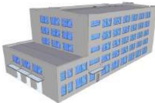
Gambar 3. 20 Ilustrasi Out-of-plane setback Sumber : (FEMA P-154, 2015)
