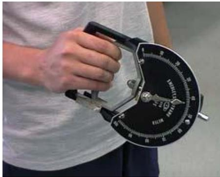
Gambar 5. Hand Grip Dynamometer
