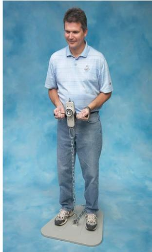
Gambar 6. *Pull and Push Dynamometer*
