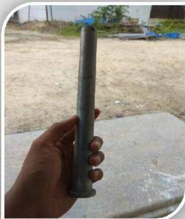
Gambar 43. Pin for vertical walling
