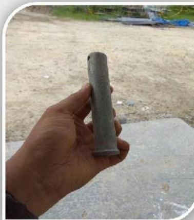
Gambar 44. Pin for *pull push prop*
